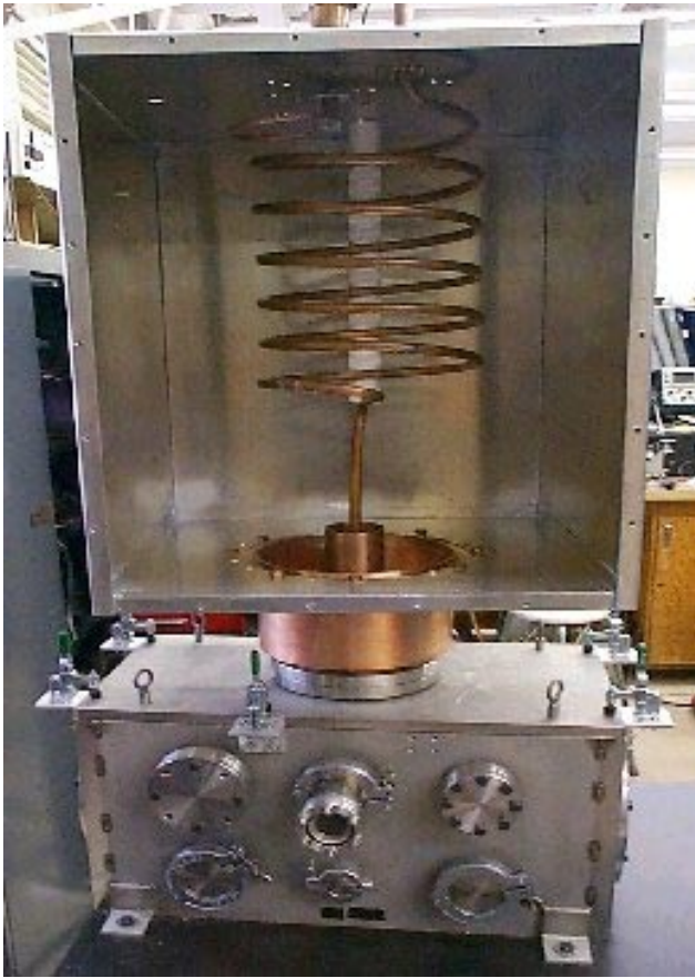
Fig. 139. The 11.9 MHz buncher prototype.
