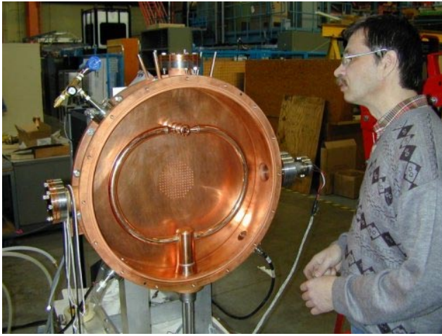
Fig. 138. One of three DTL bunchers.
