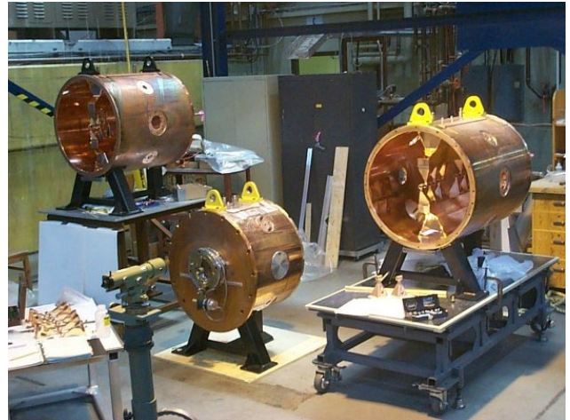
Fig. 135. DTL tanks in the assembly area.
