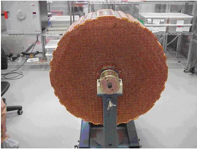
Fig. 192. Completely stacked FCAL module awaiting ground pins and anode rods.
