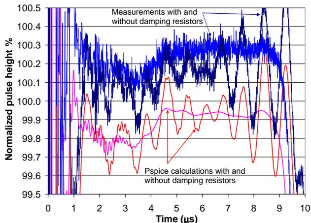
Fig. 200. PFN #2 measured and calculated pulse waveforms with and without damping resistors installed.
