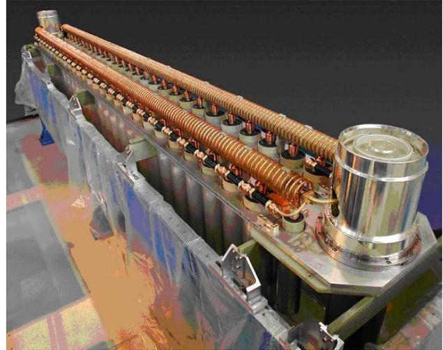
Fig. 198. One of 9 PFN under construction at TRIUMF.
