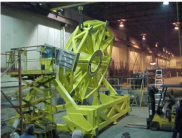
Fig. 13. Wheel rotation tooling and assembly table inside manufacturing plant in Ontario.
