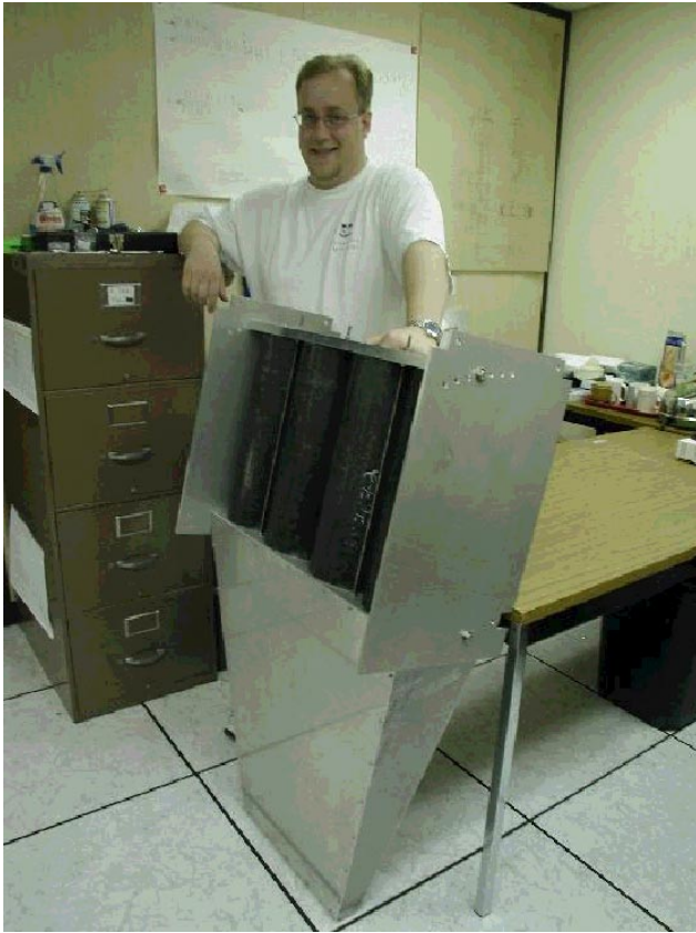
Fig. 31. Prototype aerogel Čerenkov detector at TRIUMF.
