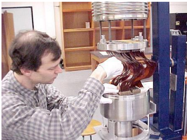
Fig. 15. Vacuum cables being installed on a feedthrough by Paul Birney (TRIUMF) at the University of Victoria.
