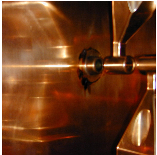
Fig. 147. DTL #3 nose cone spoiled with a soldering flux.
