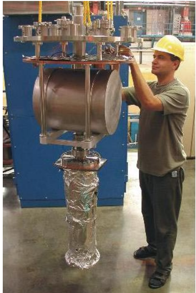
Fig. 181. ISAC-II test cryostat inner assembly with dummy copper cavity.
