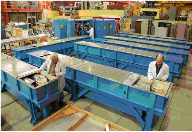
Fig. 197. Four completed RCPS and 8 PFN in storage on the proton hall roof, prior to tests.
