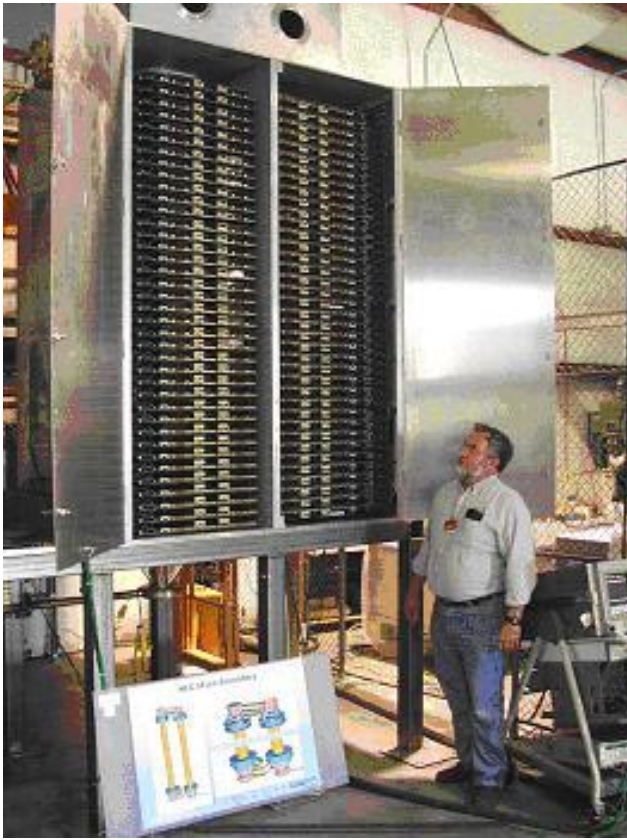
Fig. 232. Solid state induction modulator developed at SLAC.
