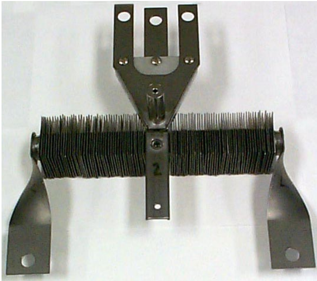
Fig. 196. Photograph of the target equipped with fins used for the heating test.
