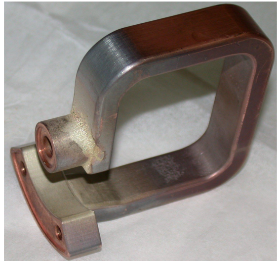
Fig. 206. Buncher #2 coupling loop with a failed soldering.
