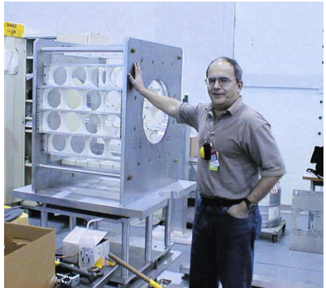
Fig. 77. CsI mounting frame during installation in the ER-2 area of Lujan Center.
