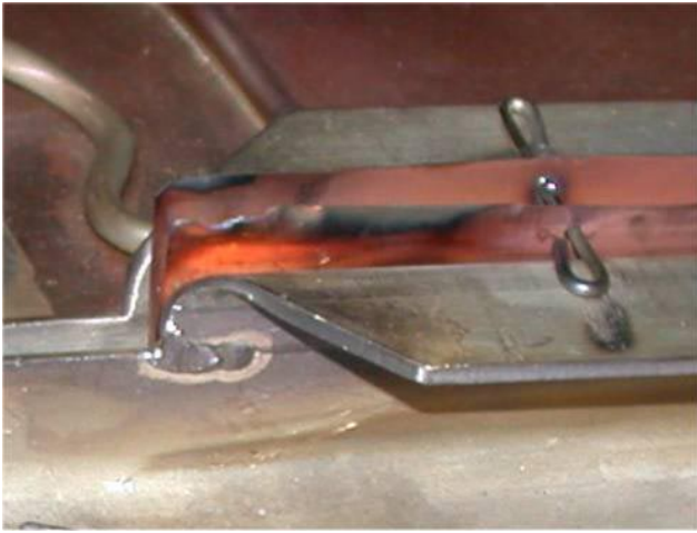
Fig. 188. Protruding M-foil, damaged by beam.
