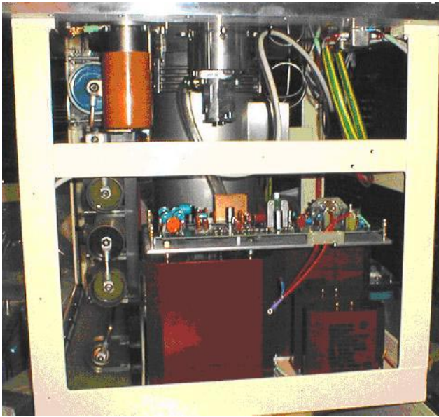
Fig. 252. One of the bias boards, without Faraday cage, cover mounted in a dump switch tank.
