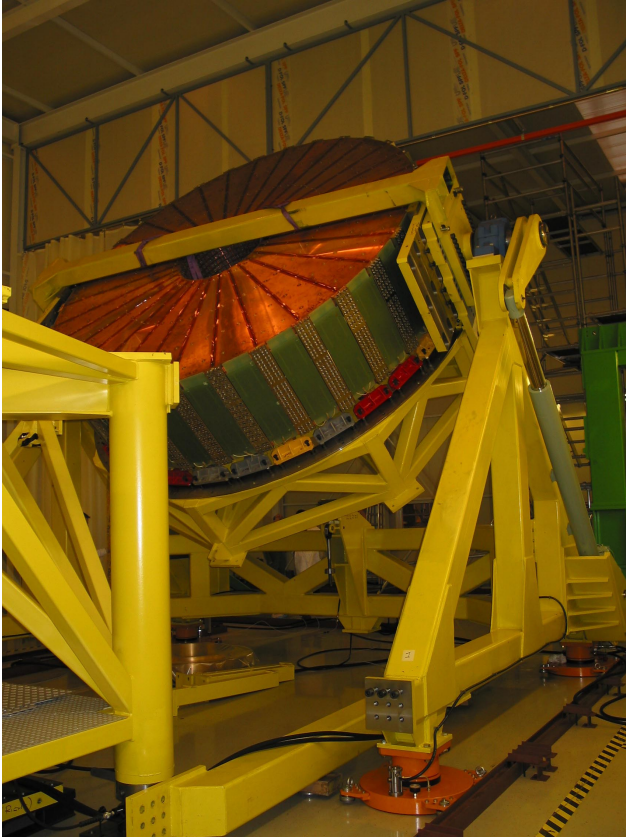
Fig. 6. First rear HEC wheel being rotated.
