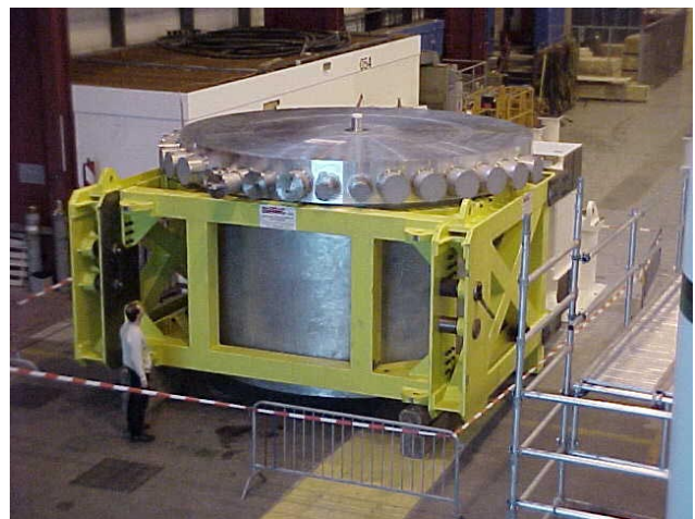
Fig. 9. The first endcap cryostat of the ATLAS liquid argon calorimeter after arrival at CERN, still in its transport cradle (April, 2002).
