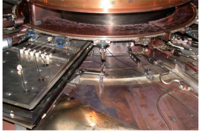
Fig. 185. View into Q1 from slightly above the median plane. The correction plate assembly is on the left.
