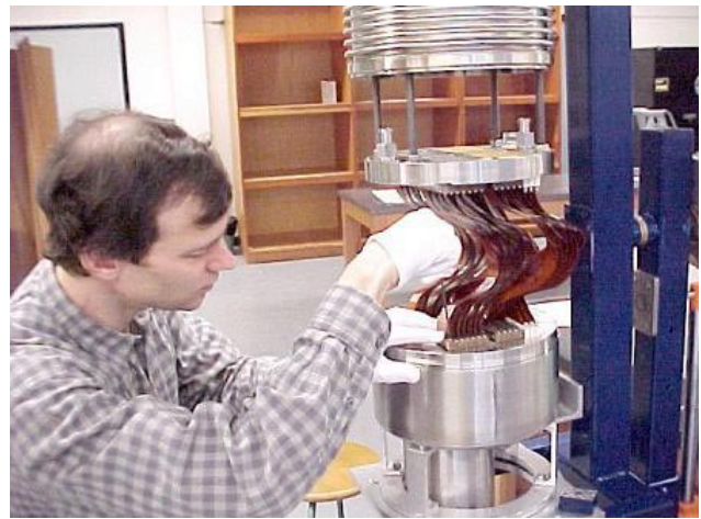
Fig. 8. Vacuum cables being installed on a feedthrough by Paul Birney (TRIUMF) at the University of Victoria.
