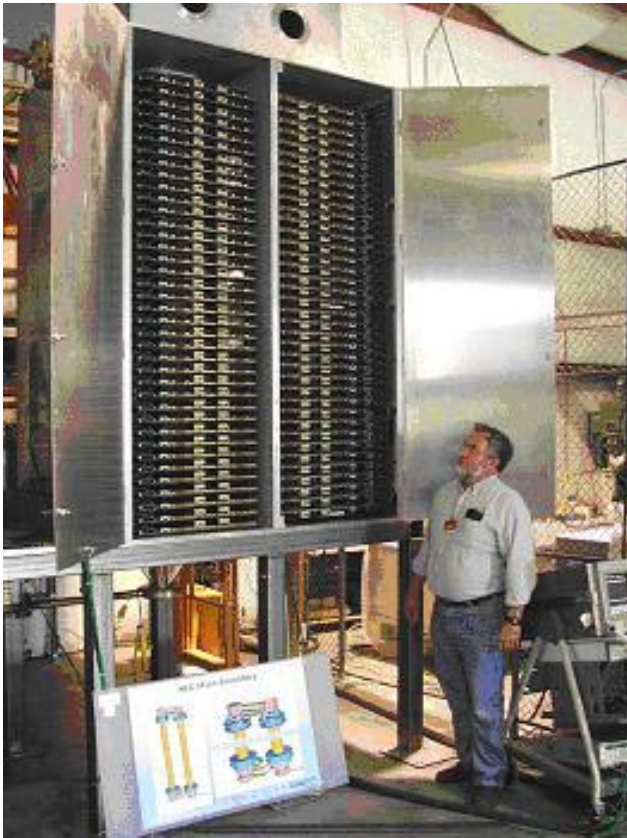
Fig. 232. Solid state induction modulator developed at SLAC.
