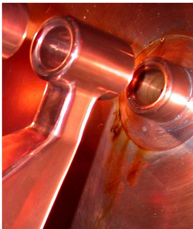
Fig. 205. Soldering flux patch in DTL tank #4.
