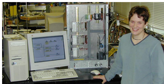
Fig. 177. PLC-based LN 2 control system in the centre, with interface computer displaying EPICS monitoring page on the left.
