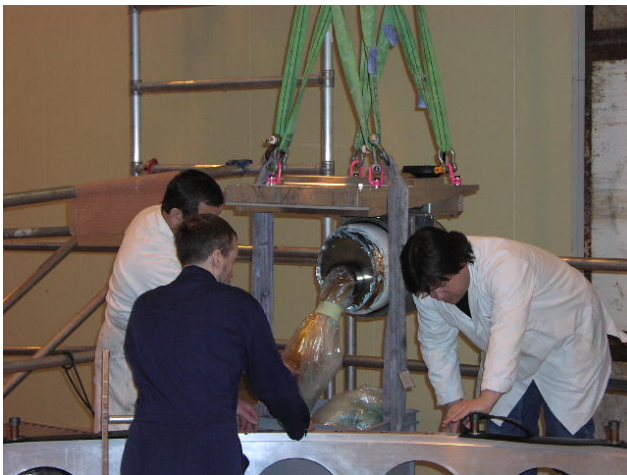
Fig. 9. Paul Poffenberger (front, Victoria) during feedthrough installation on the first ATLAS endcap cryostat.
