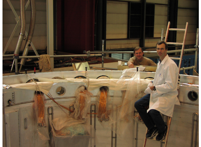
Fig. 11. Paul Birney (TRIUMF) and Ken Sexton (BNL) during feedthrough installation on the second ATLAS endcap cryostat.
