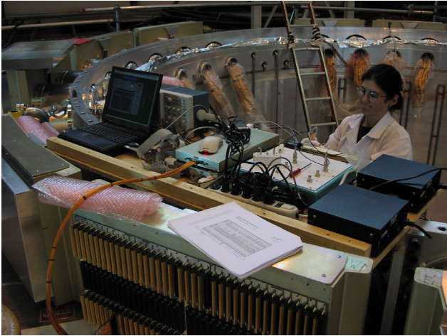
Fig. 13. Fiona Holness (Victoria) performing electrical tests on feedthroughs recently welded on an ATLAS endcap cryostat.
