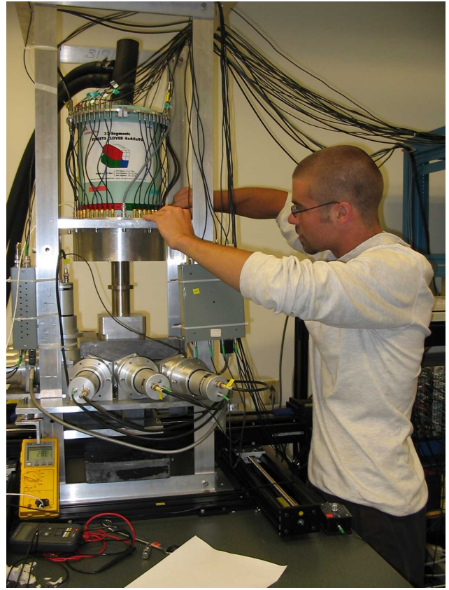
Fig. 206. Photograph of the HPGe scanning set-up being assembled by TRIUMF undergraduate scholarship recipient Nick Cowan.
