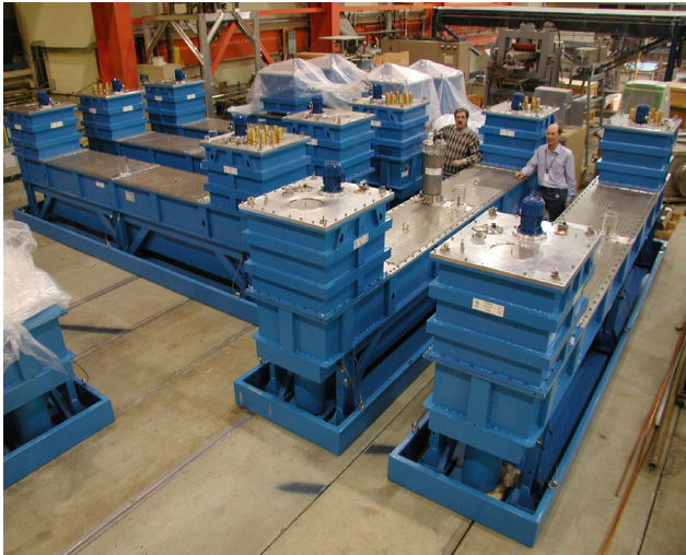
Fig. 310. 5 PFNs have been tested at high voltage and are ready to ship to CERN.
