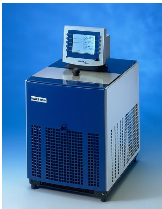
Fig. 188. A modern temperature controlled circulation system (Thermo Haake Phoenix) widely used in the chemistry program to control sample temperature from -40 to 200^{\circ}\text{C} .
