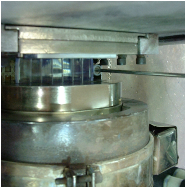
Fig. 297. Scintillator being extruded between the die and the sizer.
