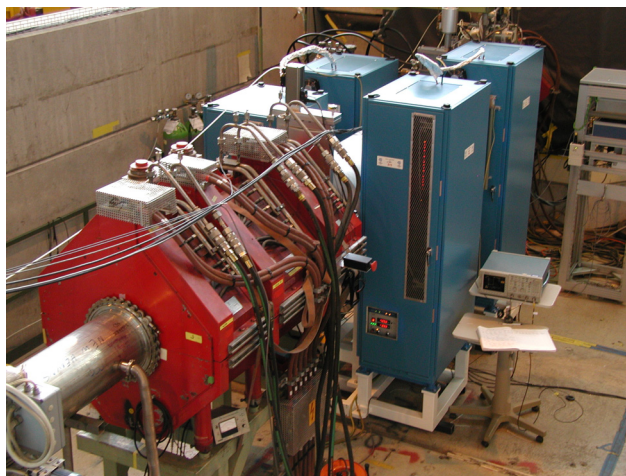
Fig. 295. MuLan kicker racks installed in beam line at PSI.
