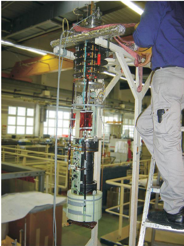
Fig. 238. ISAC-II SC solenoid in test at Accel Instruments (photo courtesy of Accel).
