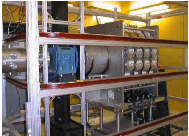
Fig. 74. CsI array mounted on the Manitoba/TRIUMF detector motion stand in the NPDGamma cave. The 1000 kg detector can be moved \pm 10 mm in x and y under computer control.
