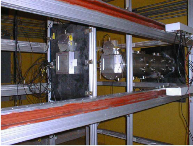
Fig. 73. Manitoba ^3\text{He} neutron monitors installed on FP12 near the start of the 2004 commissioning run. Later in the run, the monitors were used to measure neutron flux, neutron polarization, and spin flip efficiency.
