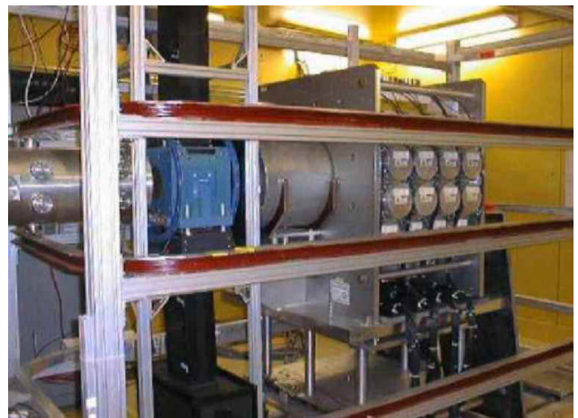
Fig. 74. CsI array mounted on the Manitoba/TRIUMF detector motion stand in the NPDGamma cave. The 1000 kg detector can be moved \pm 10 mm in x and y under computer control.
