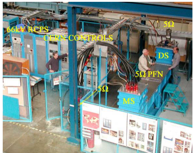
Fig. 246. PFN test set-up at TRIUMF with RCPS, and 4 CERN controls racks.
