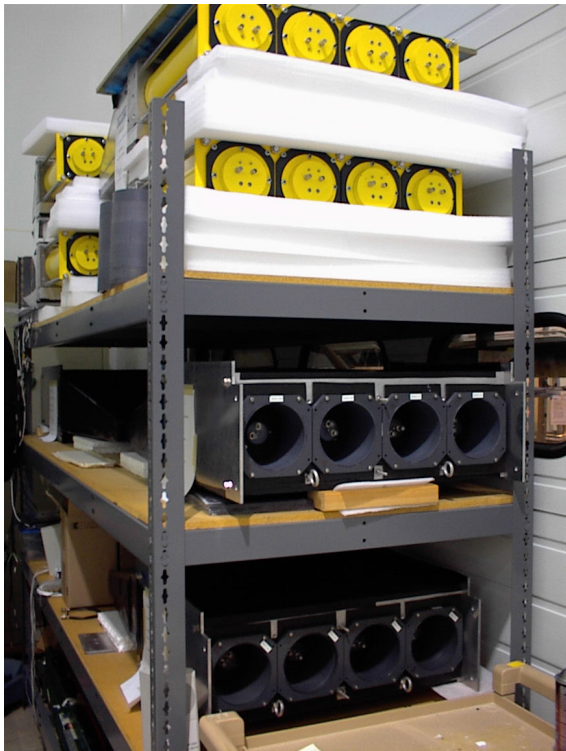
Fig. 31. The new boxes and PMT housings after arrival at Jefferson Lab and ready to go.
