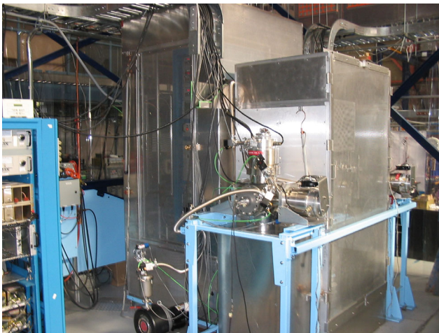
Fig. 159. The RFQ off-line test stand. Composed of an off-line source, the RFQ inside the high voltage cage, and a Faraday cup diagnosis system behind the exit, on ground potential.
