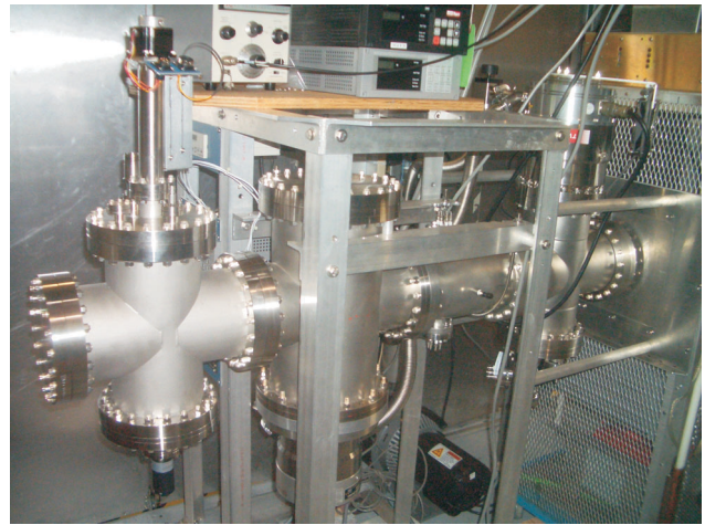
Fig. 169. Photo of the ion source test stand, with Wien-filter and emittance meter.
