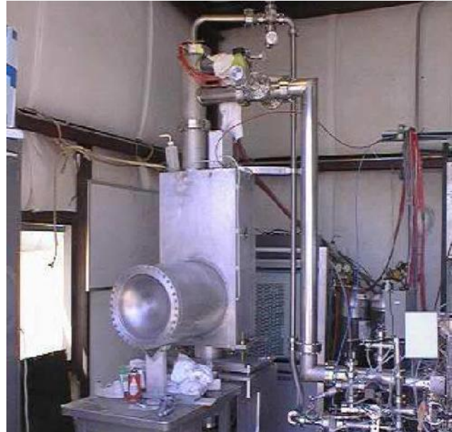
Fig. 126. Liquid hydrogen target undergoing off-line tests in the test shed. The target is expected to be installed in the FP-12 cave early in 2006.
