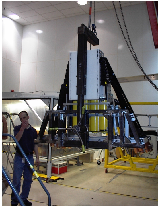
Fig. 42. A single backangle octant, complete with CEDs and Čerenkov detector installed, rotated by 180^\circ into the octant-5 orientation.
