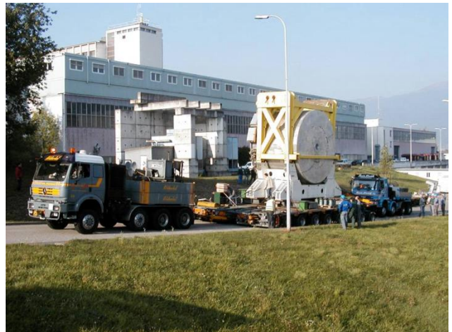
Fig. 6. Transport of the second endcap calorimeter in its cryostat to the ATLAS pit.
