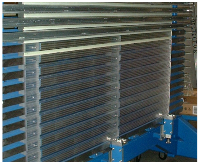
Fig. 7. Fabrication of scintillator plane. Eleven planks in the lower section have been glued.
