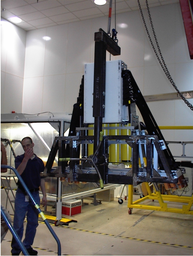
Fig. 10. A single backangle octant, complete with CEDs and Čerenkov detector installed, rotated by 180^\circ into the “Octant-5” orientation.
