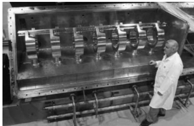
Fig. 130. Seven rings assembled, installed and aligned in the bottom section of the vacuum tank
