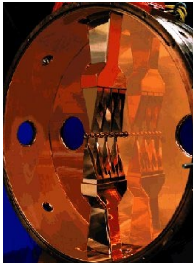
Fig. 127. The first DTL tank with the stems and ridges installed and aligned.
