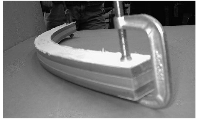
Fig. 30. Prototype CED scintillator element 2, produced at TRIUMF, sandwiched between 2 lexan guard pieces. A pair of 1.5 m long helical-bent lightguides (not shown here), also produced at TRIUMF, transport the light from the scintillator to the photomultiplier tubes.
