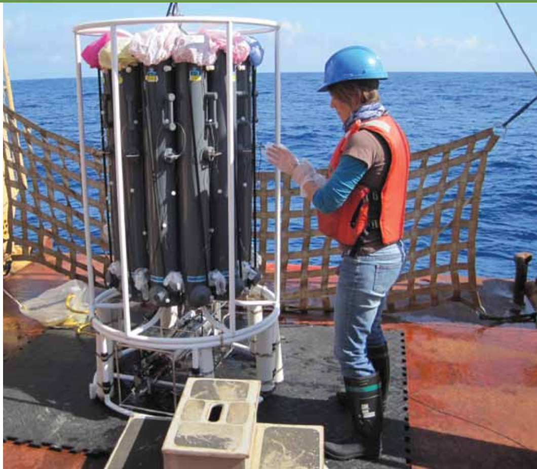
A trace metal clean rosette for sampling seawater is prepared for deployment. This rosette holds twelve 12L bottles that can be triggered to sample water at specific depths within the water column. The rosette can pick up trace levels of isotopes used in environmental science.
