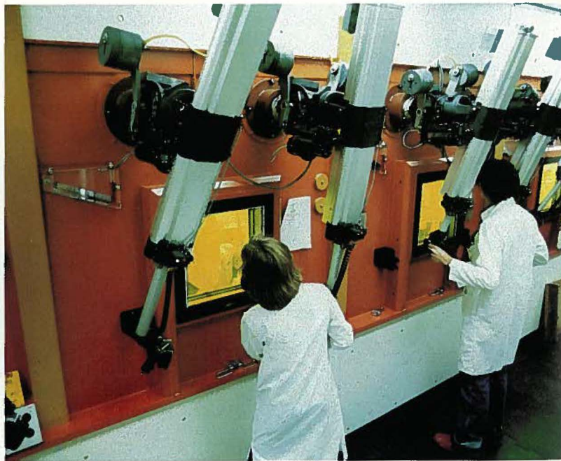
Right: Atomic Energy of Canada Limited hot cells with workers operating the remote control "hands".
