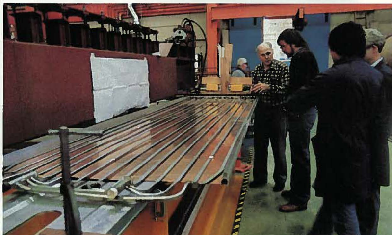
Below: Working on the prototype Radio Frequency resonator.
