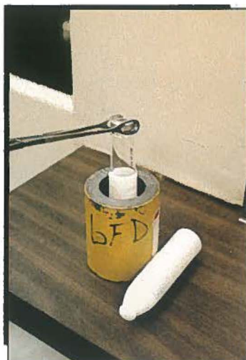
After the isotope has been incorporated into a pharmaceutical and purified, it is sealed in a vial, which is placed in a white holder—the "rabbit".
