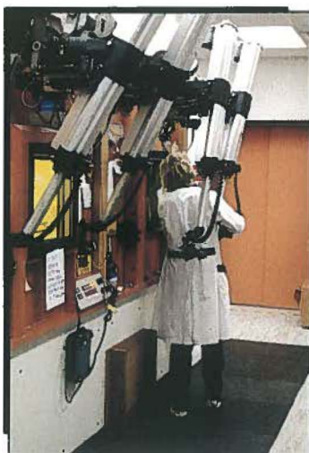
1 The targets are prepared for irradiation by operators using remote control of mechanical arms in hot cells.
