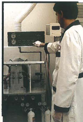
A switch is pressed, and a surge of compressed air sends the rabbit off to the UBC Health Sciences Centre, 2.5 km away. It will arrive in about two minutes, and the isotope will be used at once.
