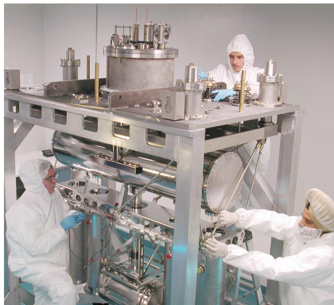
Figure 1: Soul of the new machine. TRIUMF technicians assembling one of the superconducting accelerator modules of the new ISAC-II facility.
