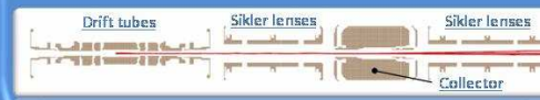
Fig. 9 SIMION simulation of the extraction of HCIs through the main components of the TITAN EBIT
