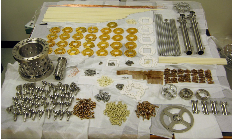
Figure A.9: Photo of disassembled CPET showing all the parts to be cleaned.
