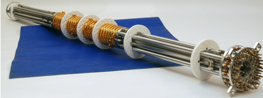
Figure A.6: Photo of the completely assembled cooler Penning trap without electrode wiring.
