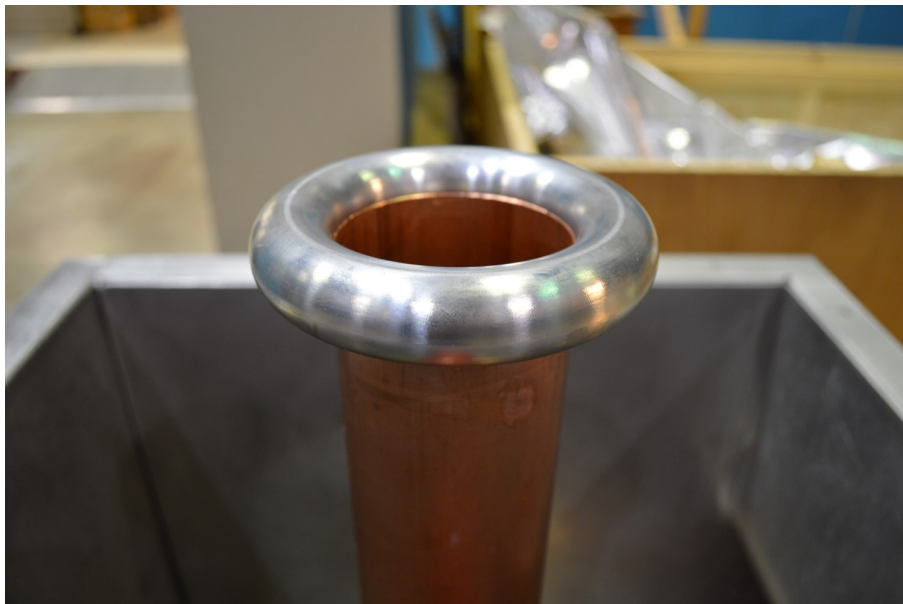
(b) Corona guard on sharp pipe end.
