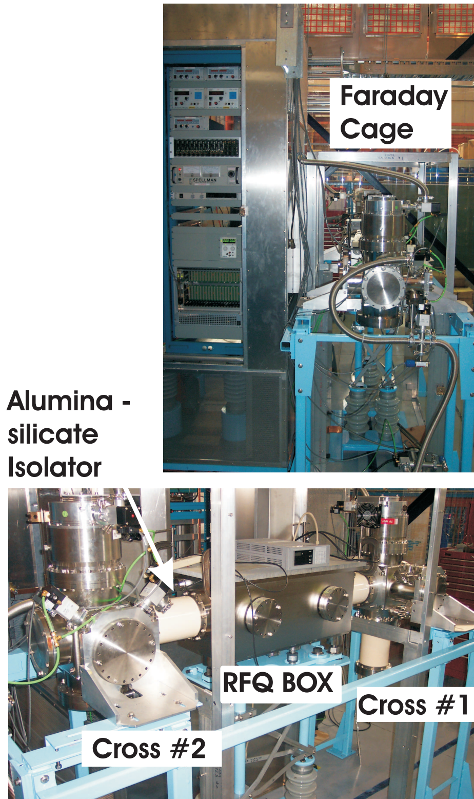
Figure 4.1: Photo of the RFQ test ion stand. The ion source is mounted on cross #1. The Faraday cage is 2.5 m tall and the RFQ box is 800 mm long.
