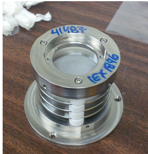
(b) Meshes installed in the holder.
