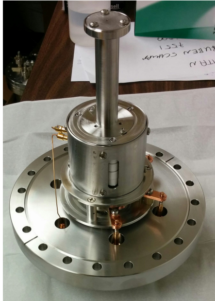
Figure 5.8: Foto of the full assembly of the used Retarding Field Analyzer (RFA). Ions, coming from the top of the picture, fly through a double hole aperture centered on the beamline axis. After passing two biased wire meshes, they impinge on an MCP detector.
