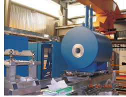
Penning trap superconducting magnet on TITAN's platform.
