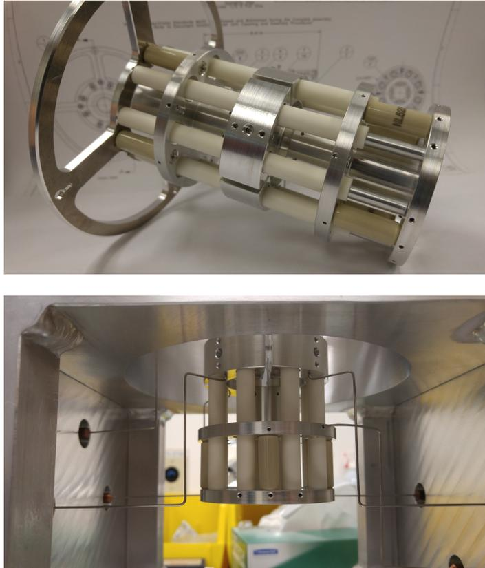
Figure 3.12: Photos of the split Einzel lens added to the TITAN beamline to facilitate high ion transport efficiency into the MR-ToF. Top: SEL prior to installation. Bottom: SEL installed in its location in the TITAN beamline.
