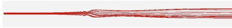
Figure 2.7: Magnetic compression of an electron beam in a magnetic field (space-charge effects are not included).
