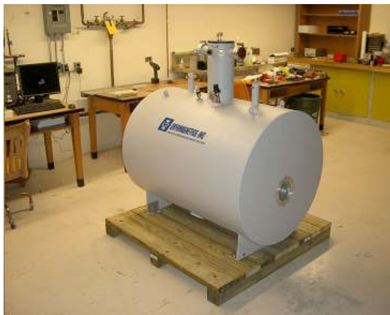
Figure 4.17: 7 Tesla superconducting magnet made by Cryomagnetics, Inc. at the University of Manitoba. The dewar has a length of 117 cm and a diameter of 86 cm.
