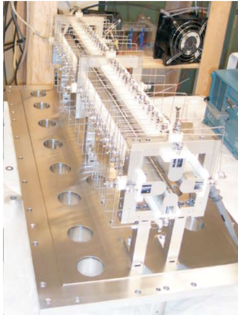
Figure 2.5: RFQ built at TRIUMF.
