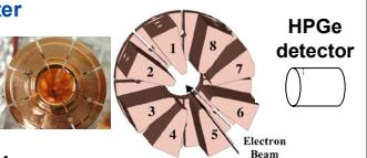
The central drift tube is segmented into 8 segments for RF cleaning of contaminants in the EBIT.
