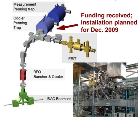
Mass measurements at TITAN with the time-of-flight ion cyclotron resonance method (TOF-ICR) can reach a precision of  $\Delta m/m < 10^{-8}$ ,  $T_{1/2} \sim 10$  ms, for short-lived radioactive isotopes (see Li-11 & He-8 Ref's.).
