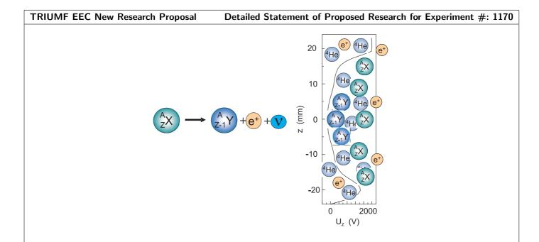
Figure 2: The beta-decay of an element. In the TITAN EBIT, employed in Penning trap mode, and filled with He-buffer gas, the recoil ions can be recaptured.
