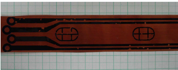
Figure D.3: After ironing the printed circuit onto the copper the transfer sheet is removed and leaves the laser-printer ink on the copper. Defects have to be covered with a protective layer afterwards with a circuit board drawing pen. After this step non-covered copper is etched off in an Iron(III) chloride-solution.
