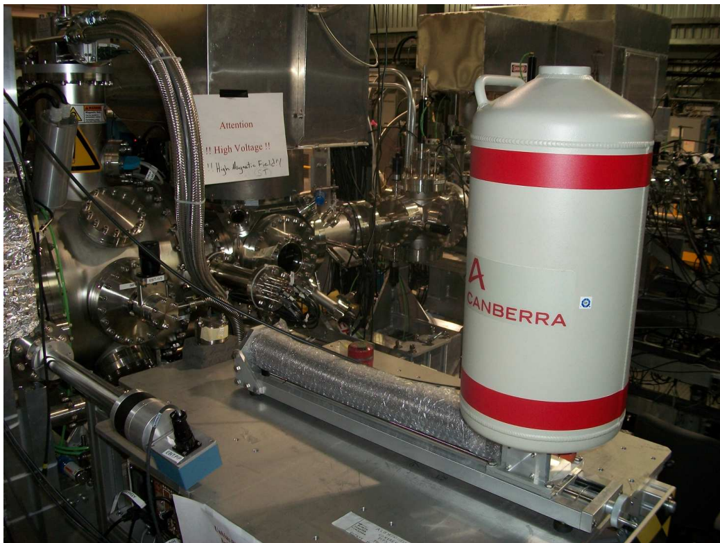
Figure 3.17: Picture of the LeGe detector prior to its installation on the North side of the EBIT.
