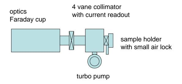
2 separate boxes for ion optics and sample stainless steel vacuum chambers with ISO or CF flanges cryo or peltier cooler if necessary only small volume for sample, easy to exchange
