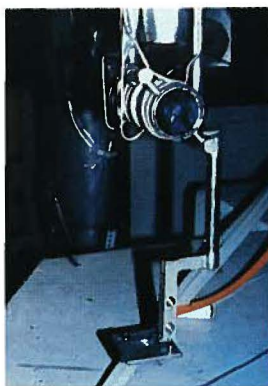
The "gas target" ready for installation in the Thermal Neutron Facility. Two radioactive gases can be manufactured at a time inside the target. The gases are piped to the Chemistry Annex where they are incorporated into pharmaceuticals for the PET program.
