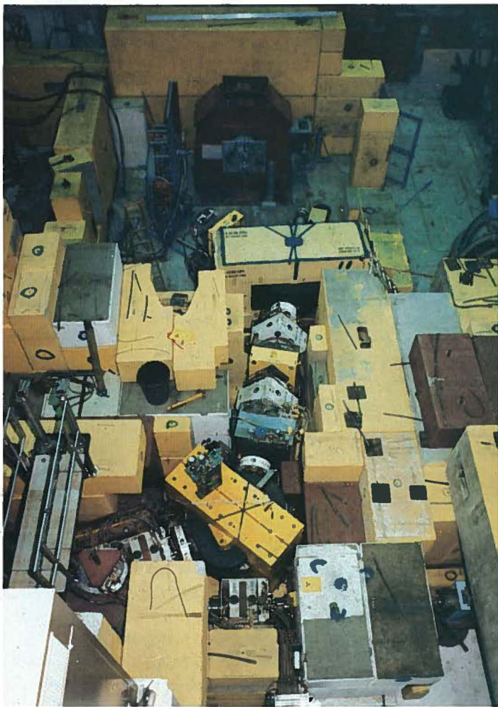
The new M11 high-energy pion channel nears completion in the Meson Hall. Nuclear physicists will soon be able to regularly use this high flux "instrument" to probe the properties of nuclei and the forces between pions, protons and neutrons. The pion production target which "feeds" the channel is at the bottom left. Pions travel down the channel (up the photo) and emerge into an area where experiments are performed.
