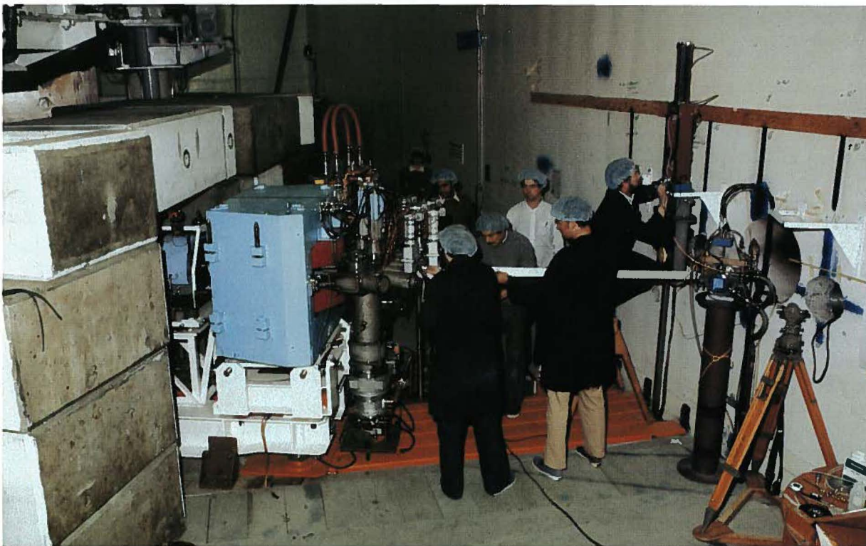
Beam line 2C nears completion in the cyclotron vault. The cyclotron (left) produces an intense proton beam which the beam line carries to the targets adjacent to the wall (right). A large (blue and red) magnet is used to select the target to be irradiated.
