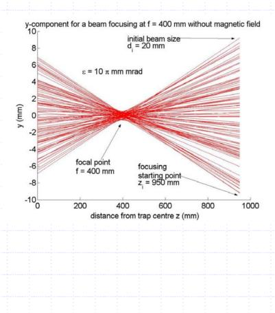
The final beam size is minimized according to three parameters before adding any optical elements: Initial beam size  $d_i$ Focal point position f Focusing starting point (einzel lens position)  $Z_i$ Other initial beam characteristics: Initial axial energy E<sub>r</sub> = 5 keV Axial energy spread:  $\Delta E = 5 \text{ eV}$ m/q ratio = 2-3 amu/e
